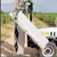
Collision protection at the rear, front and side. Aluminium clamping bar for easy re-tensioning of the fan belt and additional stabilization of the cutting unit.
